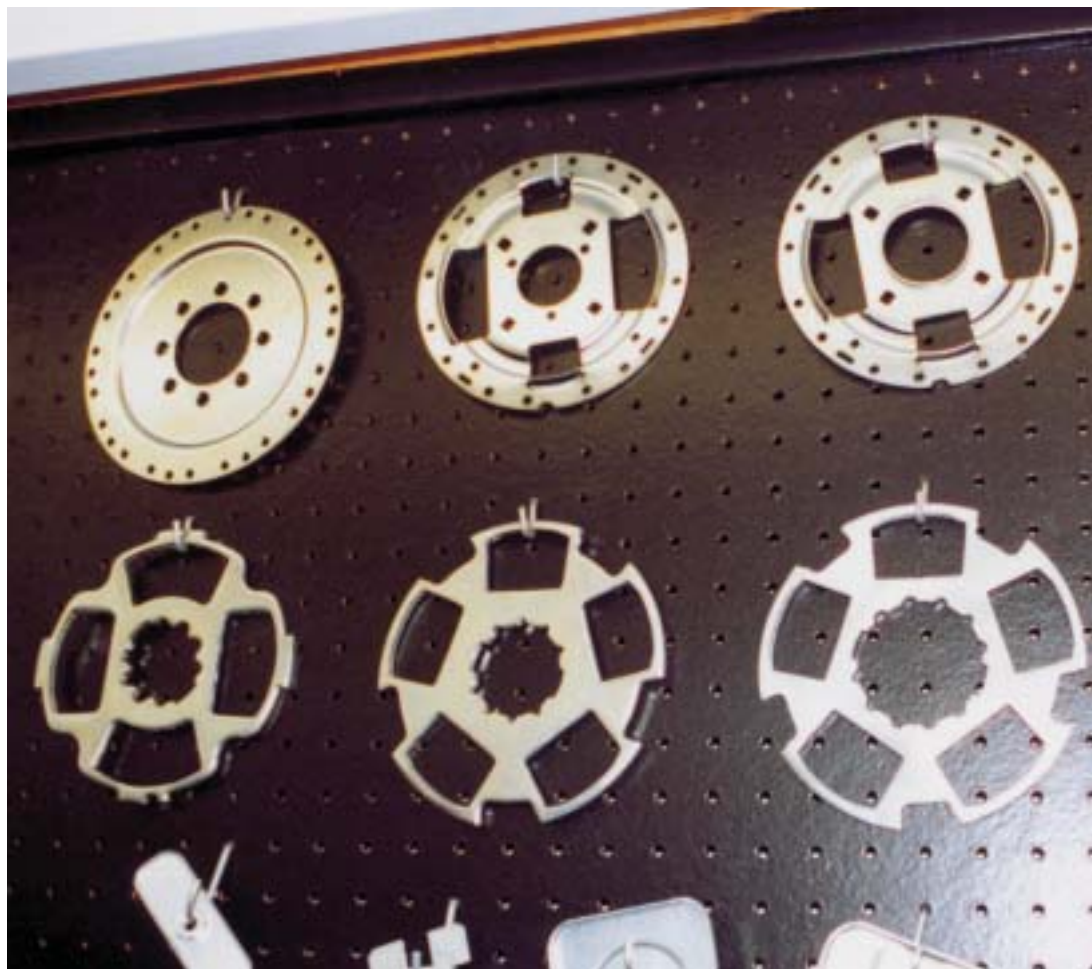
The P&G parts board includes these automotive transmission parts (middle row), some previously fineblanked by a competitor. P&G stamps them, of 5-mm-thick steel, using in-die shaving to attain the fineblank-like tolerances where needed.
